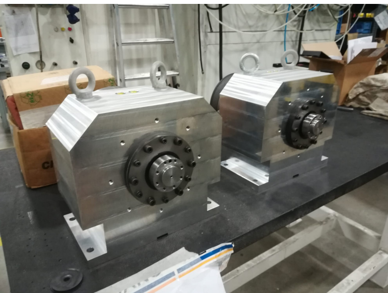
Fig. 3: gearboxes to test
