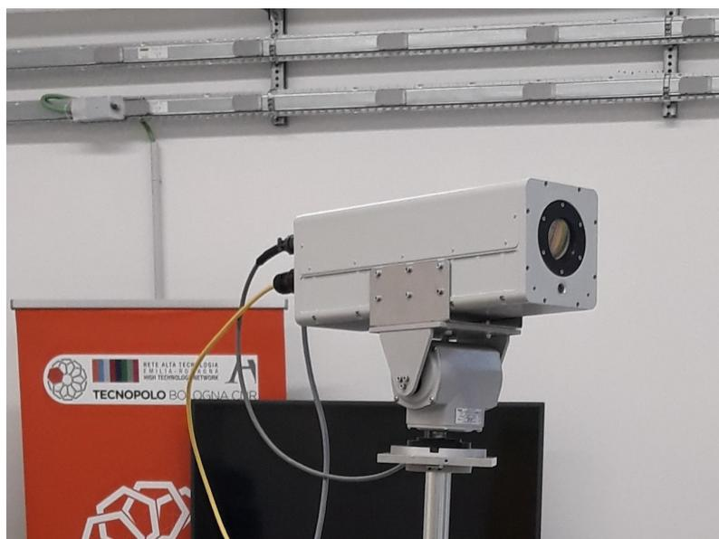
Fig. 1: QLM-1 Quantum Gas Camera
