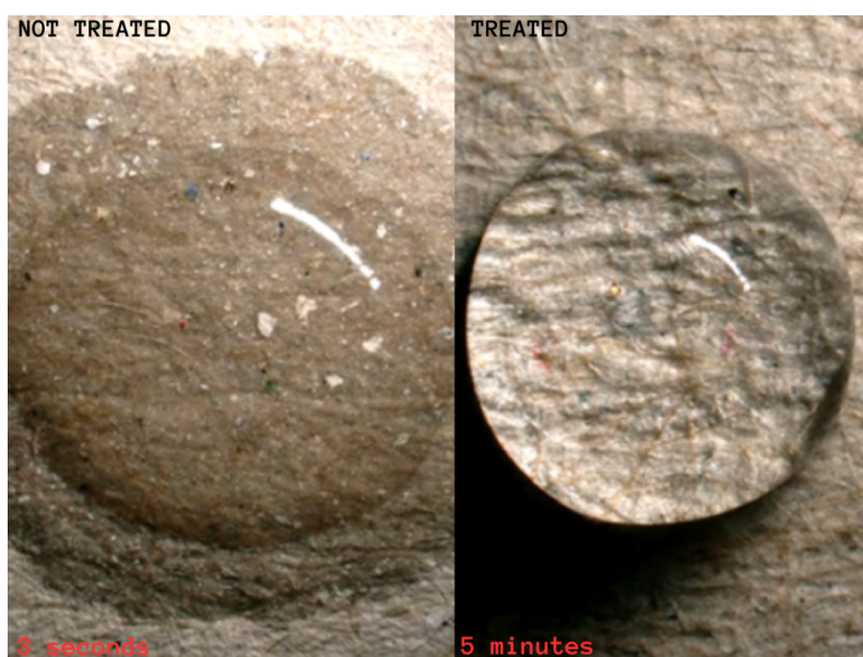
Fig. 1: Figure 1: Keyence VHX-6000 digital microscope observation of a water drop deposited on untreated (after 3 seconds) and Polysil Paper-treated (after 5 minutes) cardboard
