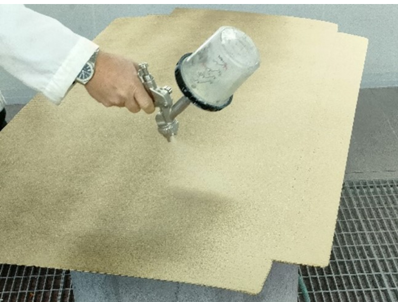
Fig. 2: Figure 2: Polysil Paper application on cardboard by spraying.
