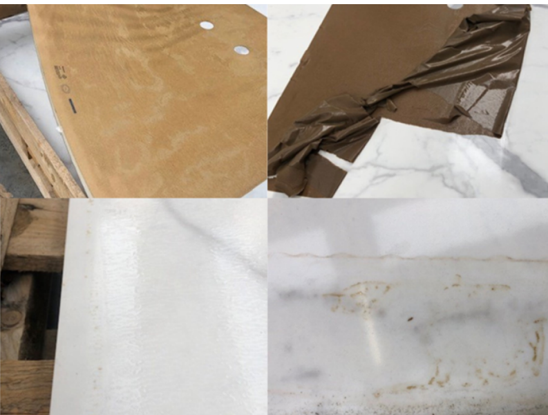
Fig. 3: Treated interlayer (upper left) vs. untreated interlayer (upper right). Slab surface in contact with treated interlayer (bottom left) and with untreated interlayer (bottom right)
