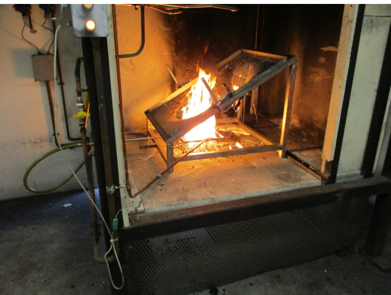
Fig. 3: R&D SBI Variation for PV4 flat roof
