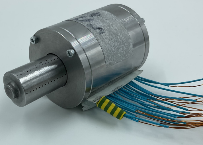
Fig. 2: First prototype of the tubular synchronous reluctance motor.
