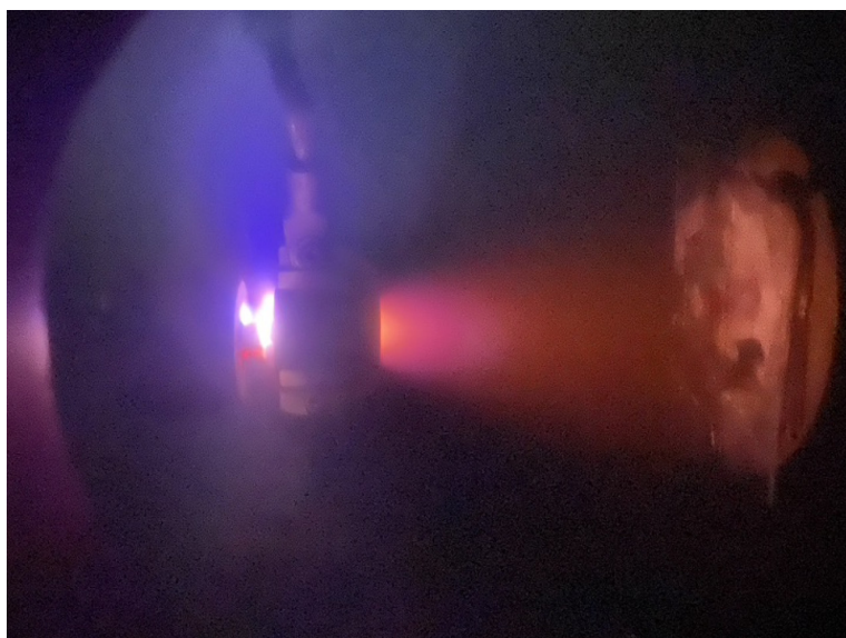
Fig. 1: Plasma plume during deposition process with the Ionized Jet Deposition System
