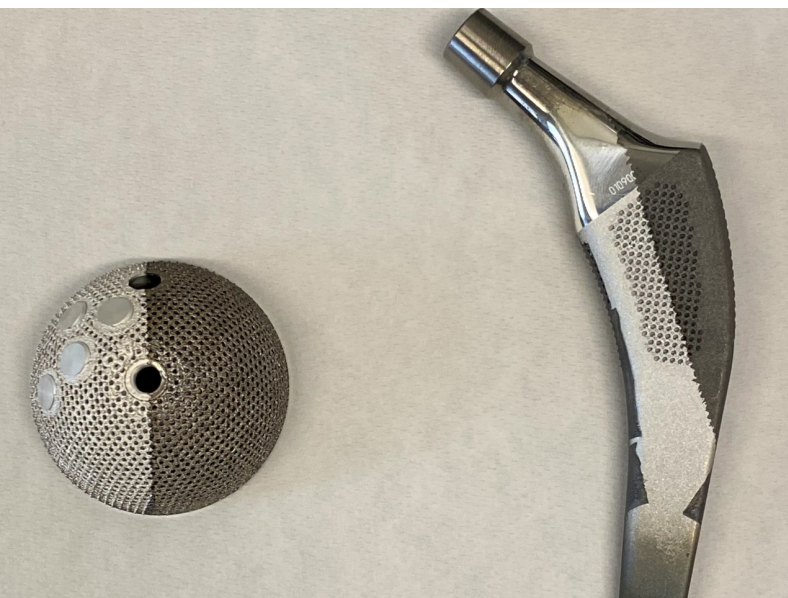
Fig. 3: Acetabular cup and femoral stem of a hip prosthesis made of titanium-aluminum-vanadium alloy, half-coated with a silver nanocoating. nio-alluminio-vanadio, rivestite per metà con nanocoating di argento
