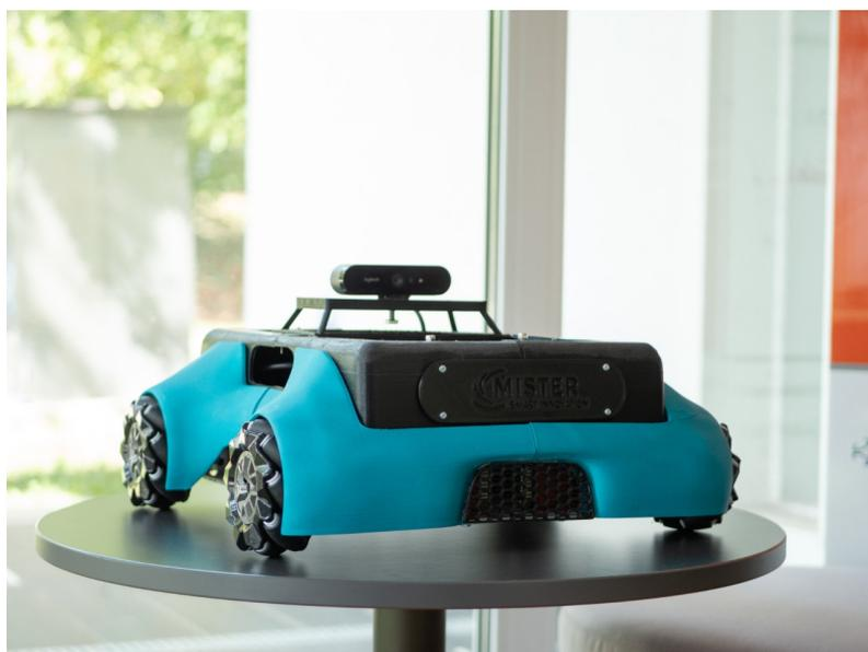
Fig. 1: MissRover AMR - Autonomous Mobile Robot
