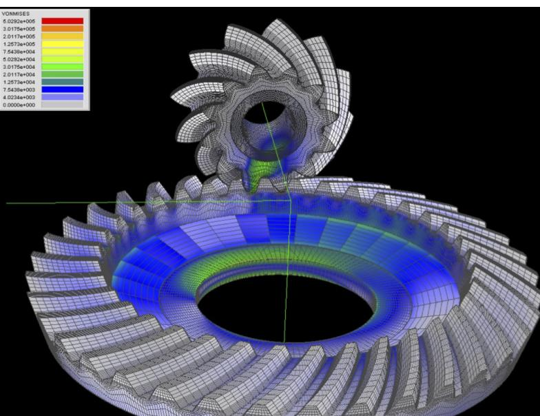
Fig. 2: FEM model of a spiral bevel gear
