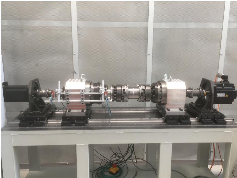
Fig. 1: test bench for servomechanisms and gear reducers
