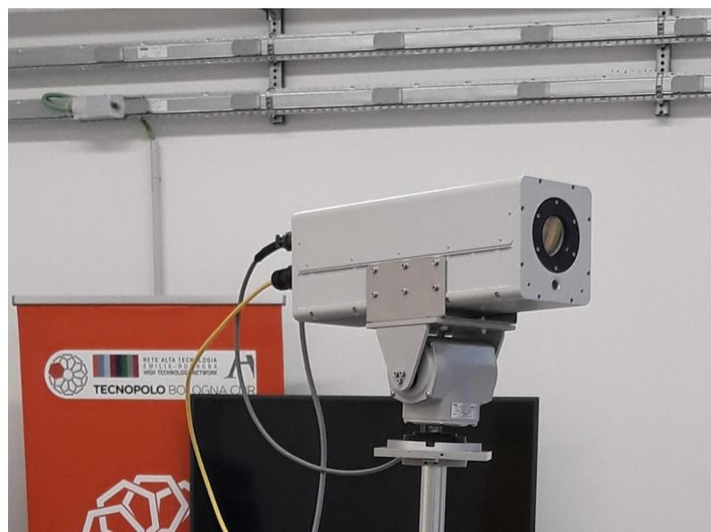
Fig. 1: QLM-1 Quantum Gas Camera
