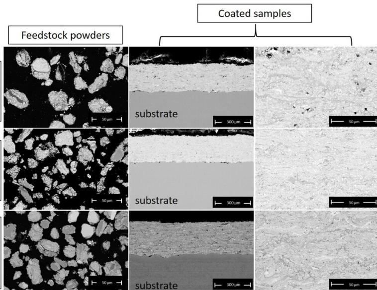
*Fig. 2: SEM micrographs of feedstock powders and of the cross-section HVOF-sprayed NbC-based coatings*
