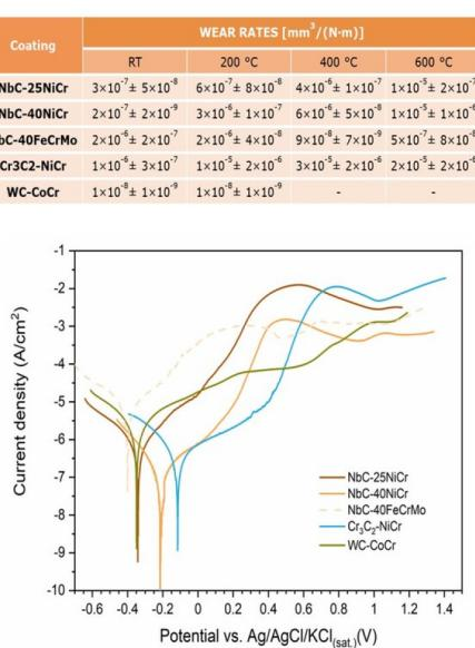
Fig. 3: Ball-on-disk dry sliding wear rates and electrochemical polarization curves of coated samples and reference coatings.
