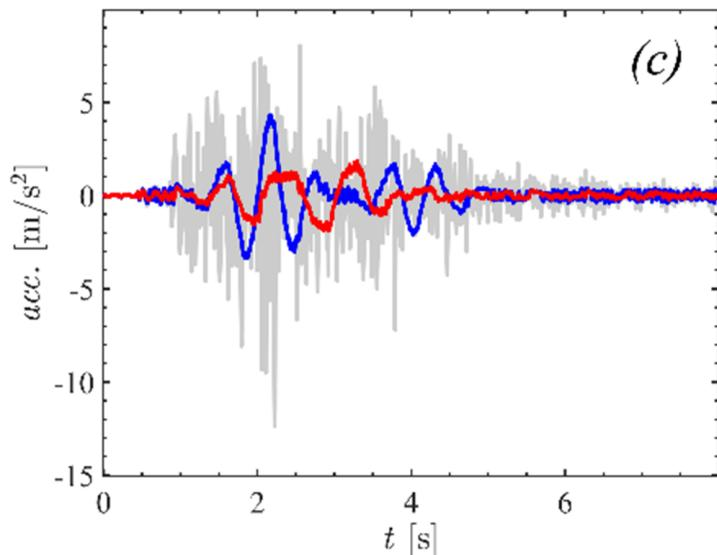
*Fig. 3: Experimental tests. Vertical acceleration time history. Bam earthquake (grey - ground acceleration, blue - Linear spring, red - HSLDS isolator).*
