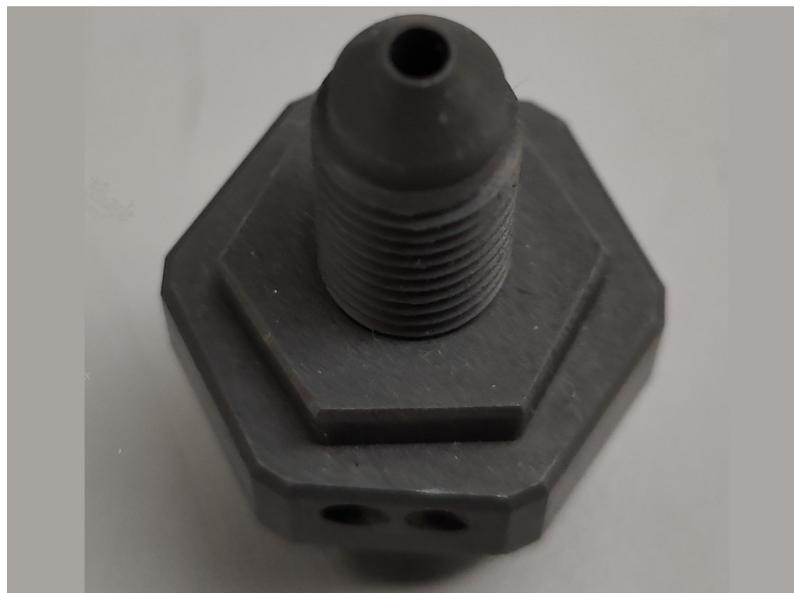
Fig. 1: ceramic filling valve
